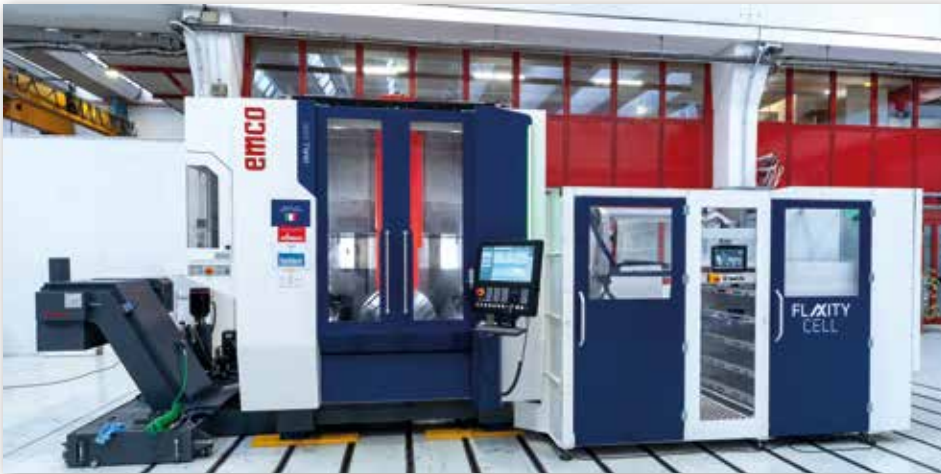
EMCO Umill 1000 universal machining center: 5-axis simultaneous machining with a portal structure.
