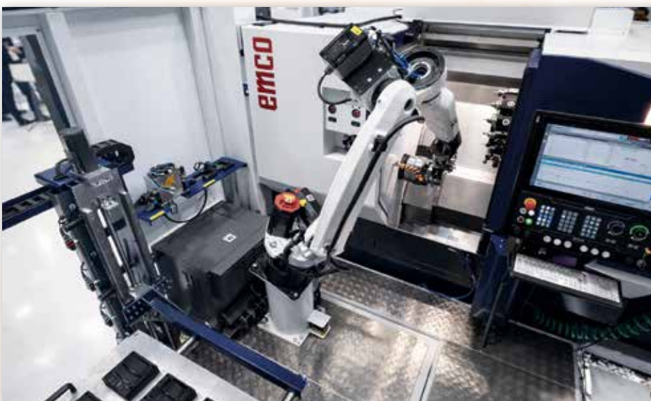
Emco Universalturm 50: The compact universal lathe for precise and efficient machining is designed for high process stability, easy operation and flexible applications in training and production.
