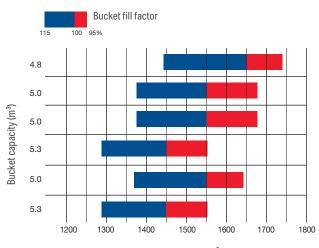
Bucket with flat bottom with teeth (C66) Bucket with flat bottom with BOC (C67) Bucket with flat bottom with teeth (C62) Bucket with flat bottom with BOC (C63) Bucket with raised bottom with teeth (C76) Bucket with raised bottom with BOC (C77)
