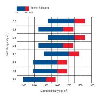
Bucket with flat bottom with teeth (C62) Bucket with flat bottom with BOC (C63) Bucket with raised bottom with teeth (C76) Bucket with raised bottom with BOC (C77) Bucket with raised bottom with teeth (C12) Bucket with raised bottom with BOC (C13) Bucket with raised bottom with teeth (Q251 + QC82) Bucket with raised bottom with BOC (Q251 + QC83)
