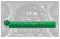
Eco guidance supports energy saving in real time (e.g. avoid long time engine idling)
