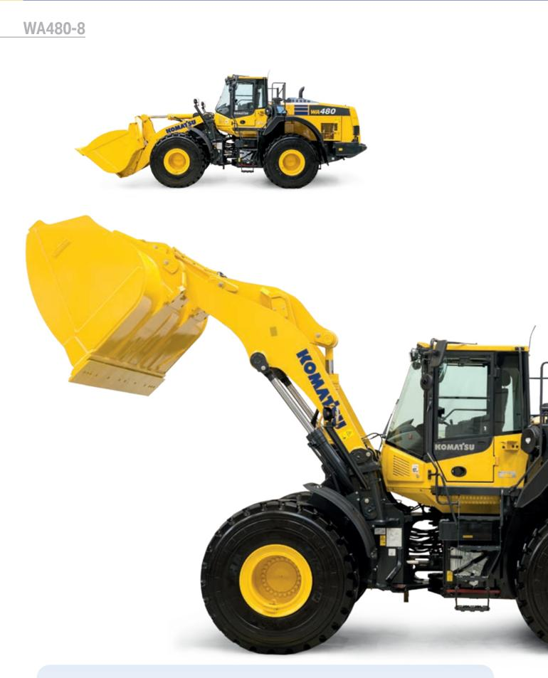
Engine power 224 kW / 300 HP @ 2000 rpm Operating weight **26315 - 27535 kg**  Bucket capacity **4.8 - 5.5 m<sup>3</sup>**
