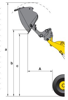
Type B, dump cylinders located outside bucket
