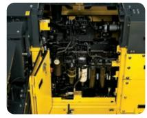
Centralised arrangement of filters
