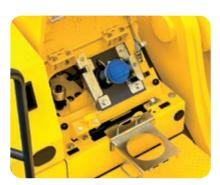
The AdBlue® tank is installed on the front stairway. The included workbench makes refilling AdBlue® even easier.
