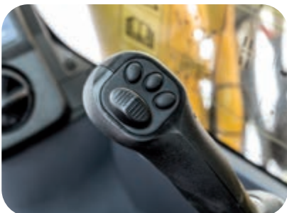
Convenient, ergonomic and precise control: joysticks with proportional control button for attachments
