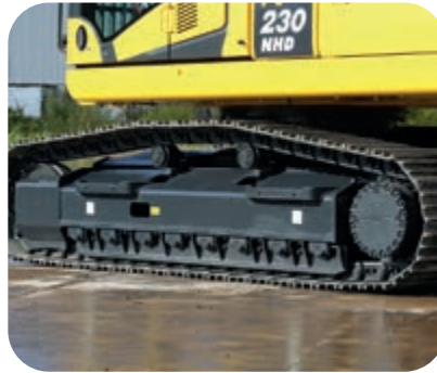
Narrow heavy duty undercarriage and narrow upper structure
