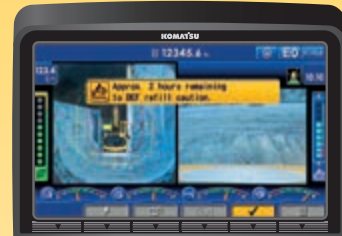
AdBlue® level and refill guidance
