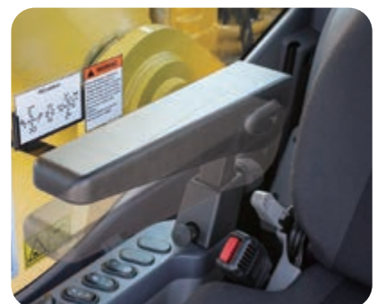
Armrest with simple height adjustment
