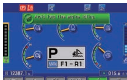
Eco-gauge, Eco guidance and fuel consumption gauge
