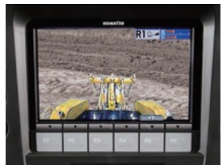
Fully integrated rear-view camera system
