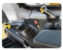
Blade control lever with auto-pitch and new ripper control lever with auto-return function
