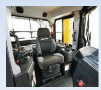
The seat is now fixed at a 12° angle to allow highest comfort for dozing and ripping
