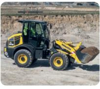
Electronically controlled suspension system load stabilizer (ECSS) (option)
