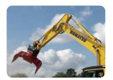
Two optional hydraulic lines to mount a variety of attachments
