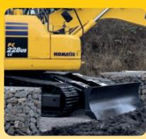
Dozer blade (option) suitable for 600 mm triple grouser (steel) and road-liner (rubber) shoes
