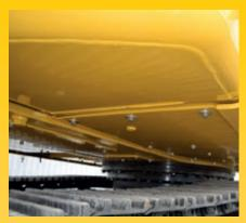
Heavy duty undercovers (9 mm) fully enclose the upper structure's underside for enhanced protection against debris on the ground.
