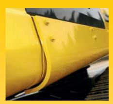
Extra heavy duty, wrap around type side protection (15 mm). Bolted to each side of the upper structure, offering protection from debris on the ground or side impact.
