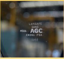
High impact protective glass (compliant with EN356 grade P5A) is fitted to front and roof window. Roof window wash/wipe system is fitted as standard.
